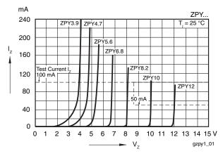
Figure 7. Breakdown Characteristics
