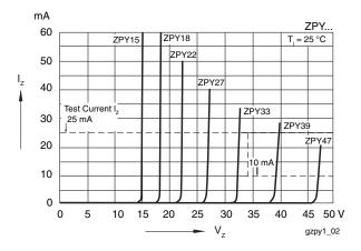
Figure 8. Breakdown Characteristics
