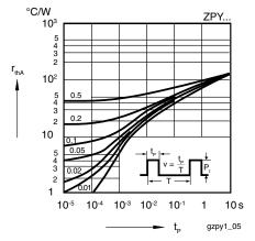
Figure 2. Pulse Thermal Resistance vs. Pulse Duration
