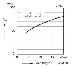
Figure 6. Thermal Resistance vs. Lead Length
