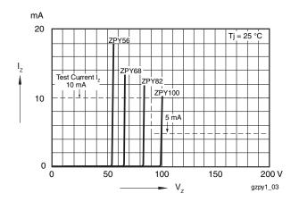
Figure 9. Breakdown Characteristics
