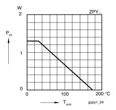
Figure 1. Admissible Power Dissipation vs. Ambient Temperature
